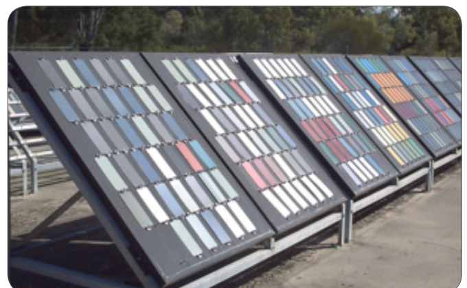
Figure 1: Outdoor Exposure – Hot Racks, Rockhampton, QLD.
