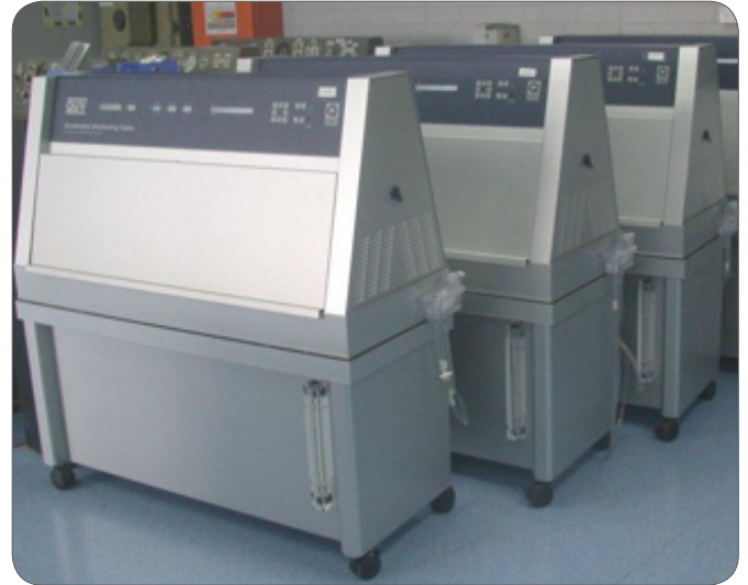
Figure 2: Hot QUVA with Solar Eye technology – used to test accelerated rates of weathering.
