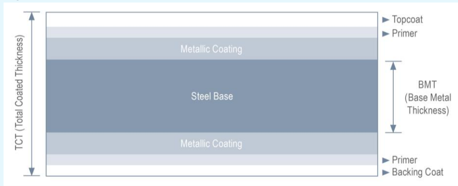
Figure 1: Schematic of BMT vs TCT for COLORBOND® steel (not to scale)
