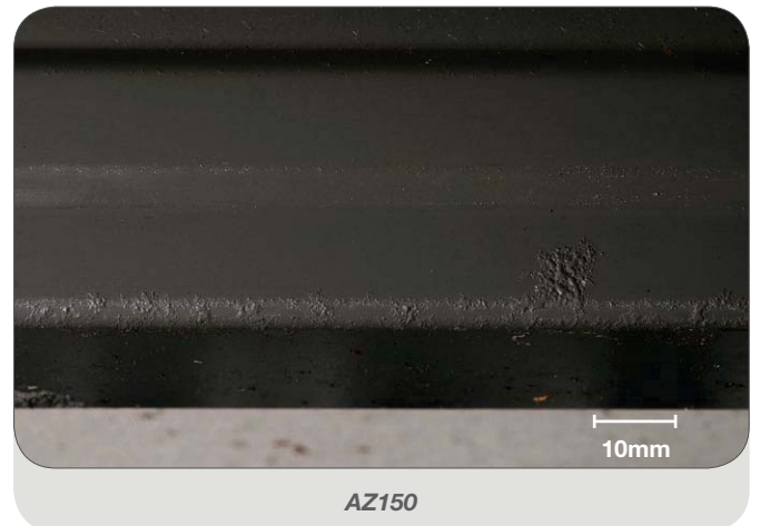
Figure 7: Prepainted, sheltered fascia bends (i.e. unwashed) after 57 months exposure within 100m from breaking surf on an outdoor test facility.
