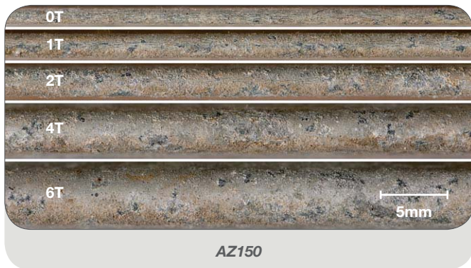
Figure 6: Unpainted samples of AZ and AM with various bend diameters, exposed in a sheltered (i.e. unwashed) severe marine environment for 45 months.
