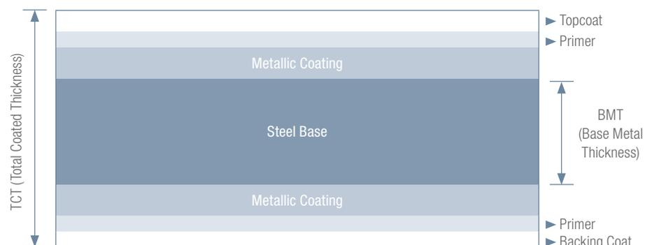
It is important to note that structural capability is a function of BMT and steel grade whereas corrosion performance is afforded by metallic coating thickness and type. Always ensure that the BMT specified is as per recommendations.
