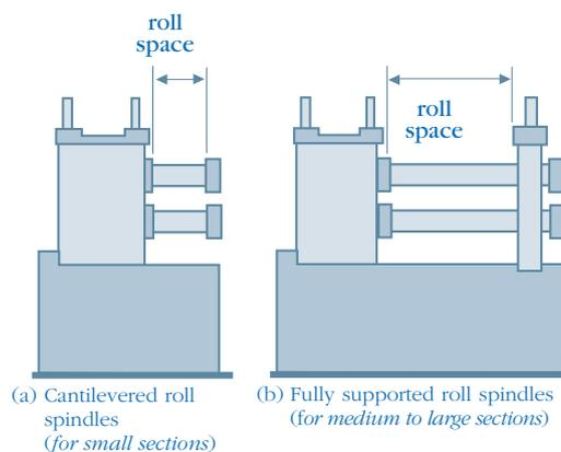
On the fully supported type, the inboard supports are fixed to the machine bed in a permanent fashion whereas the outboard stand is made easily removable for roll changing. An alternative to this is where the rolls and spindles are removed from the stands for roll changing. This requires the bridge caps to be removed and the rolls and spindles removed with a crane or other suitable lifting device.
