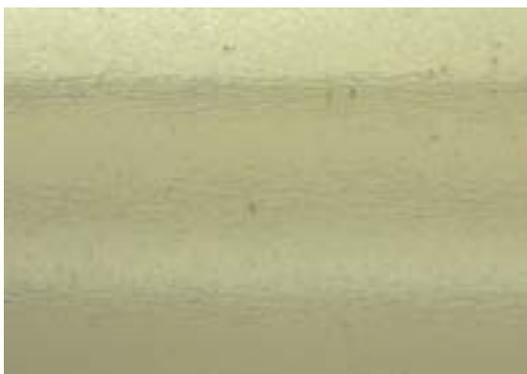
Figure 10b. - Cross section of roll formed bend (0.42mm bmt) with cracking of the paint.
