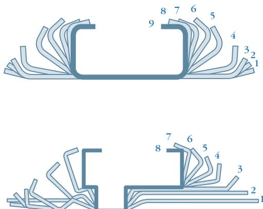
The material must be guided laterally throughout the roll-former. Initial location and subsequent guiding are provided by the entry guide, but additional guides may be required between some forming stages. Further guiding is generally carried out by the forming rolls themselves, as the portion of section already formed can provide an adequate lateral location in subsequent stages. Guiding can also be achieved by provision of locks on the periphery of rolls as shown as Figure 6.
