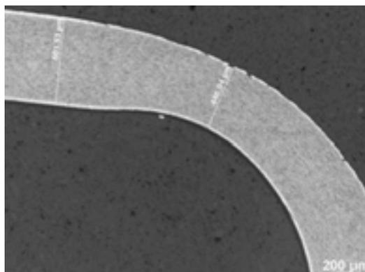
Figure 12 - Cross section of roll formed bend.
