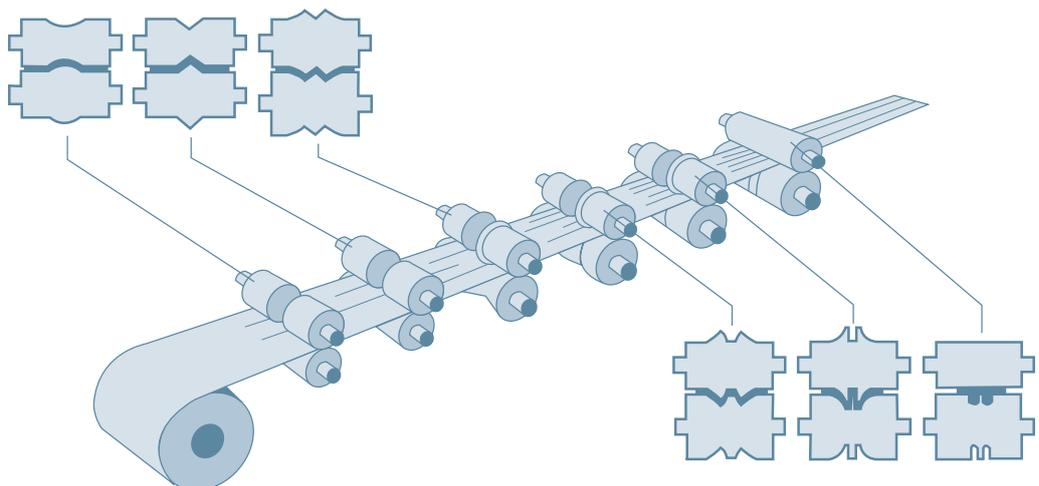
Figure 2 - Typical examples of sections produced by roll-forming
