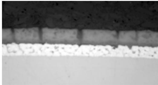
Figure 10c. Cross section of roll formed bend (0.42mm bmt) with cracking of painted and metallic coatings.
