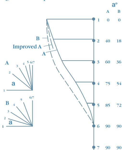
Figure 8 shows that sequence A is preferred because it gives a much better exit than sequence B. Sequence A may be improved if a is reduced slightly in stage 2.
