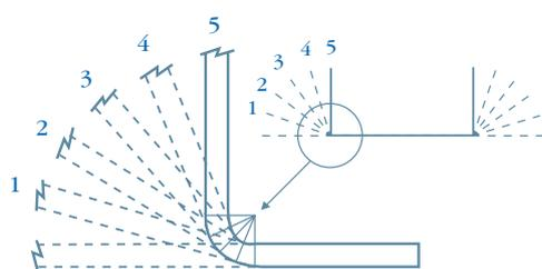
(a) Conventional forming of ductile steels
