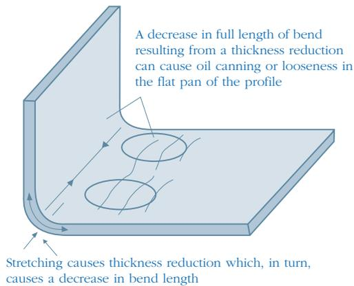
Top spindle rolls should be checked for proper mating with the aligned lower roll profile. A thin, flat strip of feed material or feeler gauges can be used as a gauge to ensure that feed will have sufficient clearance to pass between the mating roll profiles and not be subjected to ironing which may locally stretch the material and cause oil-canning, edge wave or rippling.
