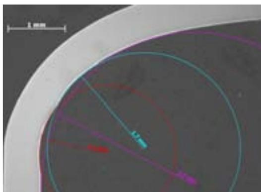
Severe bend thinning will significantly reduce the strength of the base metal and may result in splitting and/or other defects of the material.
