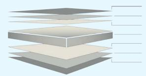
Finish Coat (Finish Coat + Primer = nominal 33µm) {Refer Notes 1, 5 & 6} Universal Corrosion Inhibitive Primer
