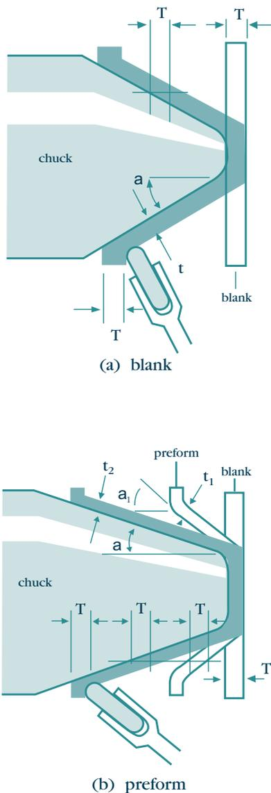
When  $a$  is outside the range of 13 to 80° the feasibility of shear forming should be seriously considered. Below 12° thinning and metal working are excessive, beyond 80° the blank becomes unstable.
