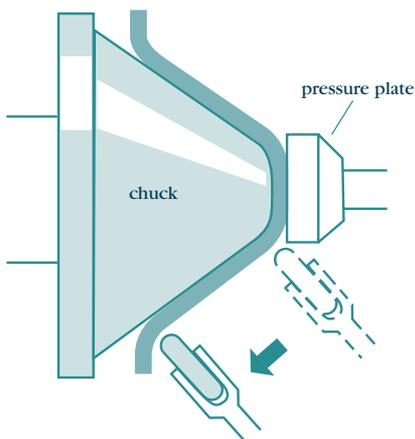
Flow forming is an elongation process for reducing the wall thickness of a thick-walled cylindrical preform to produce a cylindrically shaped final product.
