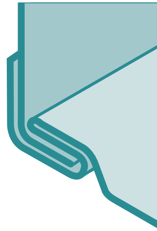
Figure 2 - Completed Pittsburgh lock-seam
