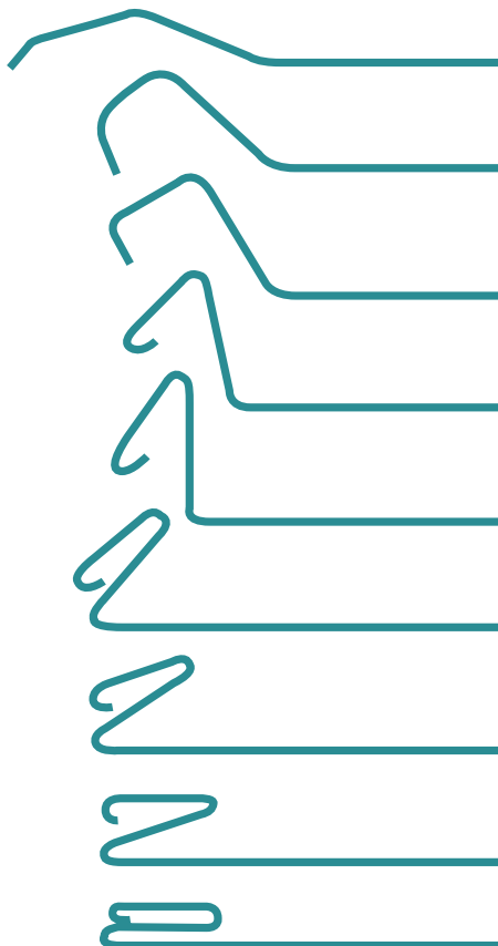
Figure 4 – Button Punch Snap Lock formation stages
