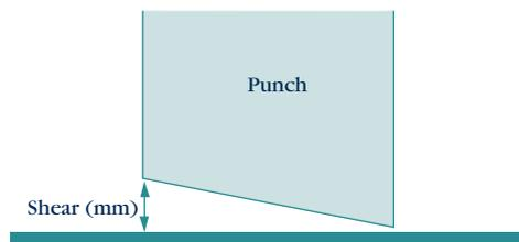
In general, angular shear equal to 33% of stock thickness reduces shearing force by approximately 25% and shear equal to stock thickness, or full shear, reduces shearing force by 50%<sup>2</sup>. Shear is not usually used with slender punches as they lack column strength. In this case, a similar reduction in maximum load can be achieved by staggering the punch length in compound tools.
